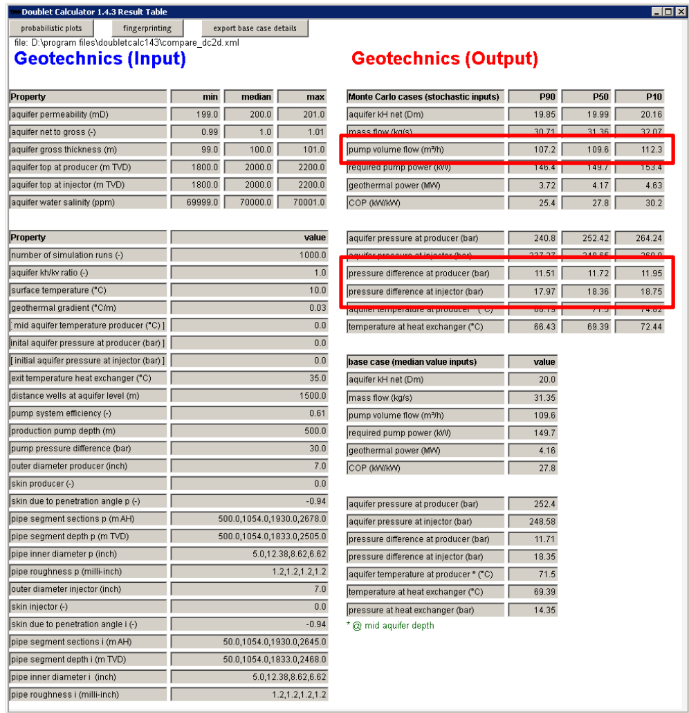
Figure 15 DoubletCalc results screen showing flow rate and pump pressure difference (compare to Figure 18).
