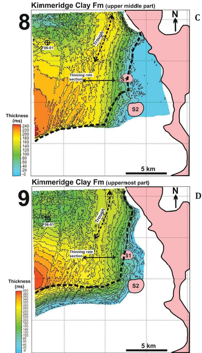
Figure 16 A-D. Isopach maps of Units 6-9, representing the Kimmeridge Clay Fm, and showing similar thickness distributions. Apart from the W-E thinning at the margin zone, radial thinning can be observed in the northwest that creates a NE-SW oriented trough in the north in case of each unit. In Unit 6, a local bowl form can be observed in the east adjacent to the salt wall, similar as of Unit 5.
