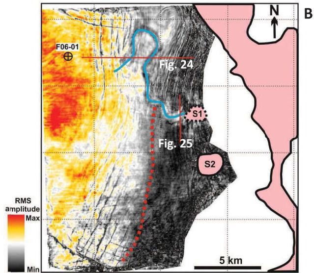
Figure 23. A-B. RMS amplitude map from base Middle Graben Fm in Unit 3 depicts linear amplitude pattern in the north of the study area. The feature shows rapid bends at the basin margin in contrast with the sinuous bend of 2 km radius in the basin axis. Red lines indicate cross sections of Figures 24 and 25. Dotted red line indicates N-S oriented boundary between high and low amplitudes, which correspond to prominent stratal termination at Base Middle Graben Fm (Unit 3) in Figure 19.
