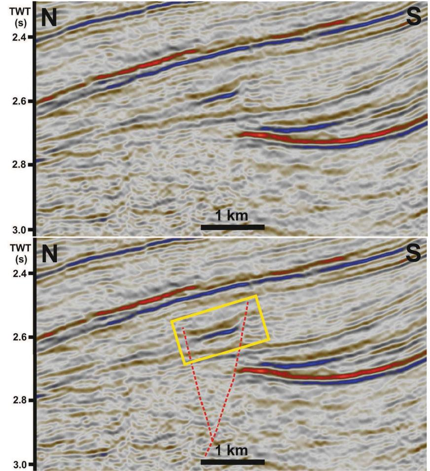
Figure 25. N-S cross sections showing 2-D seismic representation of linear amplitude feature (yellow rectangle) of Figure 23. The high amplitude zone is bounded by elevated flanks.
