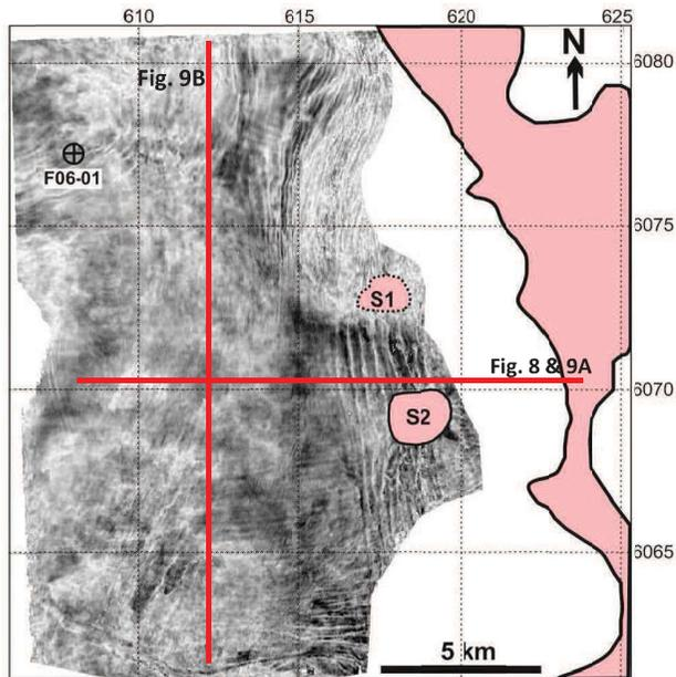
Figure 7. RMS amplitude map of intra Unit 1 horizon in the lower part of Lower Graben Formation depicting fault pattern at the basin margin in the proximity of the salt bodies. Faults are oriented N-S and radially from salt body 2. Note the higher number of faults in this map in the Lower Graben Formation and their minor occurrence in the younger Kimmeridge Clay Formation (Figure 6).
