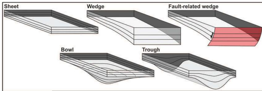
Figure 10. Stratigraphic external forms of growth packages. From Bouroulec et al. (in press)
