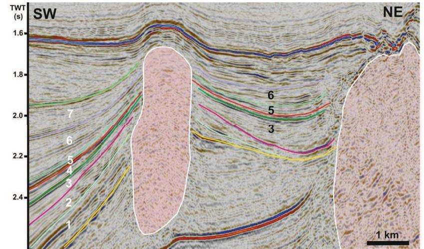
Figure 20. Cross section highlighting the wedge external form of Unit 3 and local thickening trends in units 5 and 6. See location in Figure 13.
