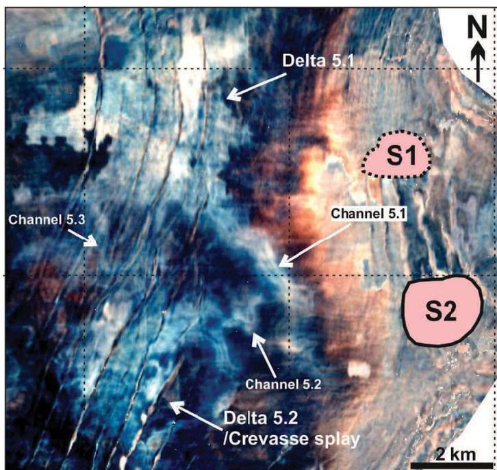
**Figure 38.** Color-blended spectral decomposition map from the upper part of Upper Graben Formation (Unit 5), highlighting linear elements terminating in well-defined delta-like or circular zones.
