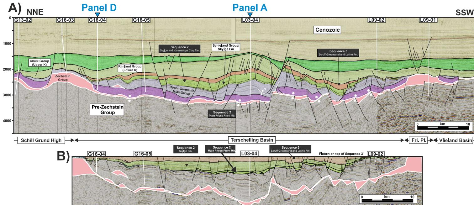
Panel B1 is located across four structural provinces, namely from north to south, the Schill Grund High, the Terschelling Basin, the Friesland Platform and the Vlieland Basin. This panel trends NNE-SSW and is composed of four figures. See Fig. A4.1 for location map and Fig. A4.2 for legend.
