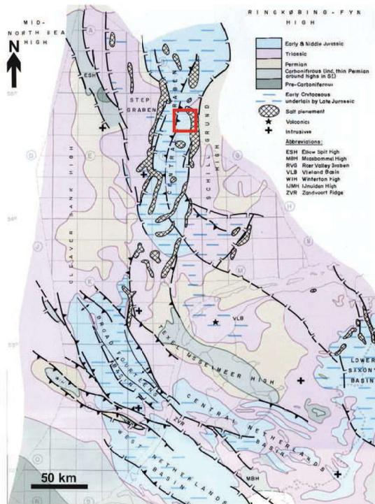
**Figure 3.** Basement fault trends, salt structures, and the distribution of Upper Jurassic sediments in the Dutch offshore. The salt wall, located in the east of the study area, follows the north-south trend of a major basement fault, bounding the Dutch Central Graben. The study area is marked by red. (from Van Wijhe, 1987)
