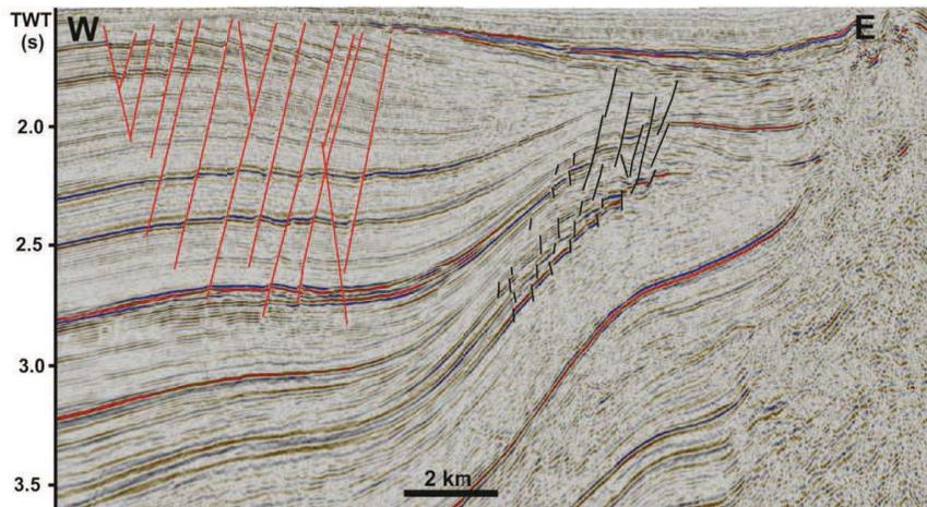
Figure 8. E-W seismic cross section with some interpreted basin axis (in red) and basin margin faults (in black) in 2-D cross section from the middle of the study area (see Figures 5-6 for location), (5x vertical exaggeration)
