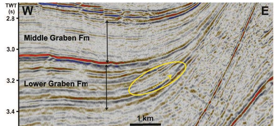
Figure 30. W-E cross section showing a distinct zone of discontinuous seismic facies in the Lower Graben Formation (yellow circle). The discontinuous zone is underlain by a clearly truncated reflector (yellow arrow).
