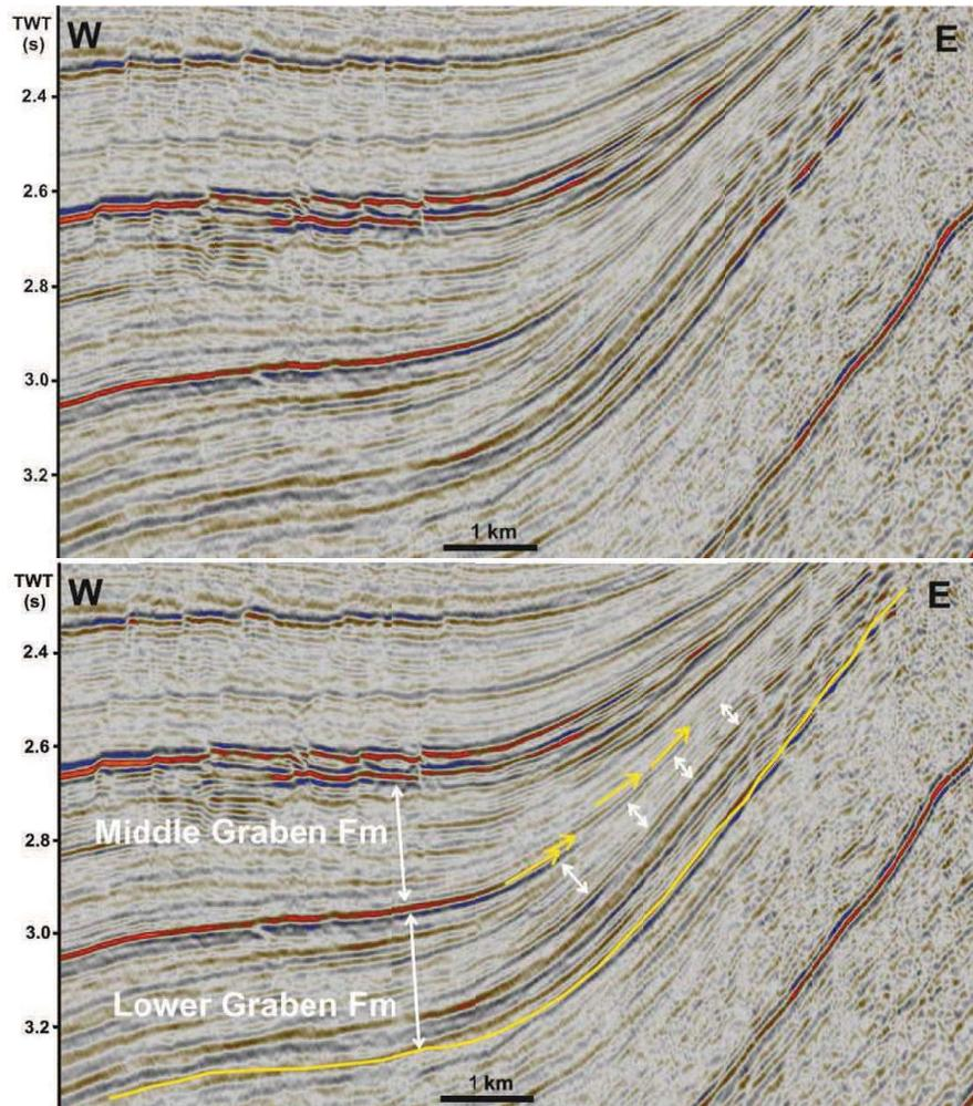
Figure 19. Terminating reflectors in Unit 2, 3 and 4, in the Middle Graben, and Lower Graben formations in the middle part of the study area. Note low rate of thinning in Unit 2, upper part of Lower Graben Formation. (white arrows)
