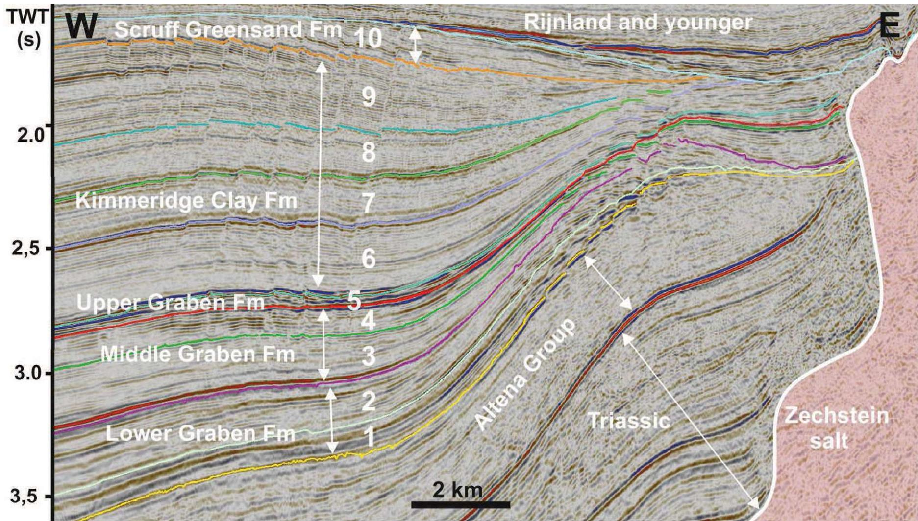
**Figure 9 A.** Characteristic W-E seismic cross section (5x vertical exaggeration) depicting the seismic signature of the Upper Jurassic in the Middle of the study area with stratigraphic subdivision in this study (1-10) and corresponding formations. See **Figures 6-7** for location.
