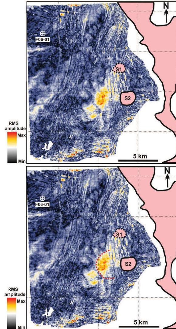
Figure 32. Sweetness attribute map from base Unit 4 in the Middle Graben Fm depicting high amplitude radial pattern at the margin-axis transition, west from salt body 1. Outline is plotted on Figure 41. 4 isopach map.
