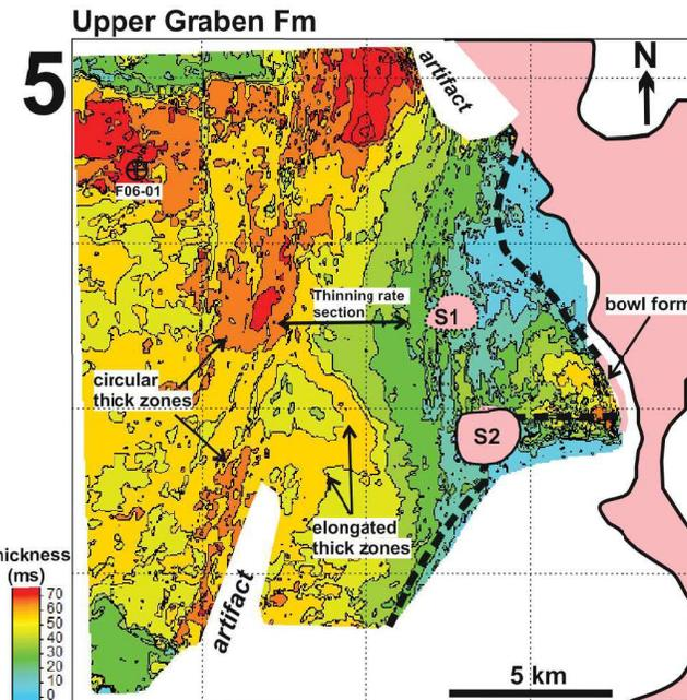
**Figure 15.** Isopach map of Unit 5, representing the Upper Graben Fm. Locally thickening can be observed between the salt wall and the salt bodies creating a bowl external form. Prominent reflector terminations are marked by dashed and dotted lines. Pink zones depict the basin bounding salt wall and allochthonous salt bodies S1 and S2, pink line refers to direct contact with salt wall.
