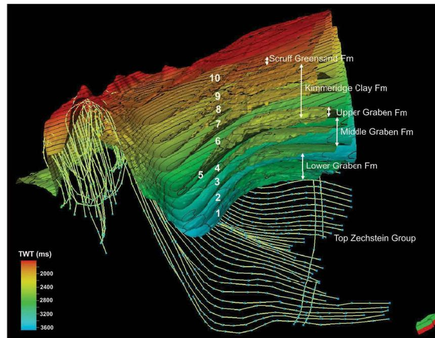
Figure 5. Three-dimensional display of the 11 interpreted horizons, which define the stratigraphic units (1-10) used in this study, along with the corresponding formations (arrows), and the Top Zechstein Group.
