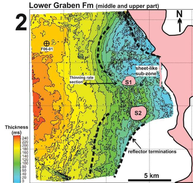
**Figure 12.** Isopach map of Unit 2 representing the Upper part of Lower Graben Fm. The main thickness trend is thinning towards the margin. Note very low rate of thinning between the two salt bodies that creates a sheet-like sub-zone. Prominent reflector terminations mapped and marked by dashed and dotted lines. Pink zones depict the basin bounding salt wall and allochthonous salt bodies S1 and S2, pink line refers to direct contact with salt wall.
