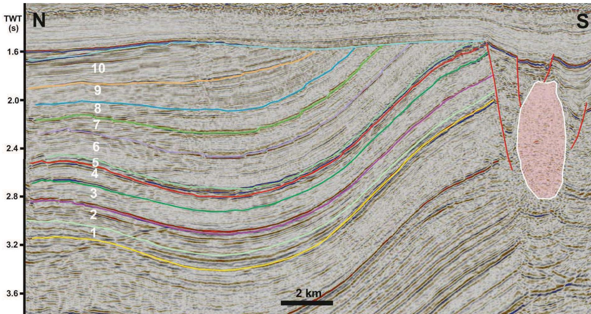
**Figure 9 B.** Characteristic W-E seismic cross section (5 times vertical exaggeration) depicting the seismic signature of the Upper Jurassic in the middle of the study area, with stratigraphic subdivision in this study (1-10) and corresponding formations. See **Figure 7** for location
