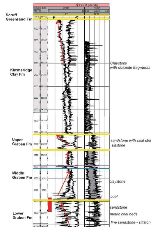
Figure 2. Gamma ray and sonic log response of F-06-1 well, located in the northwestern part of the study area, see Figures 6-7 for location, The well does not penetrate through the whole Upper Jurassic but its deepest reach lies within the Lower Graben Formation. Red arrows indicate coarsening (towards the left) and fining (towards the right) upwards grain size trends.
