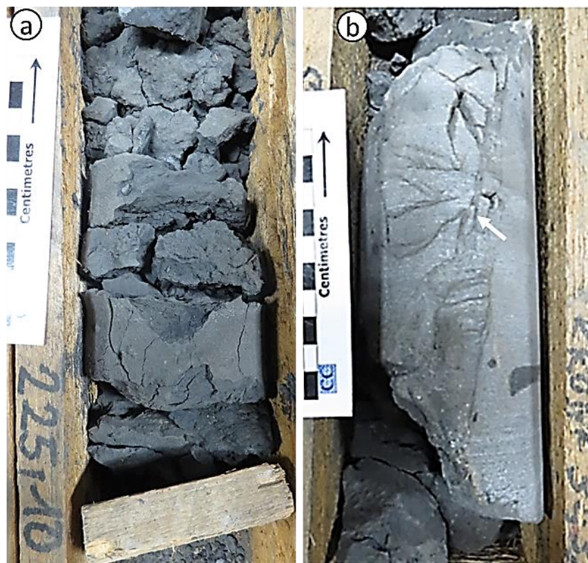
Figure 6-39: a) Dark grey powdery mudstone, HEU-01, 225 m. b) Fractures in basinal Dinantian carbonate mudstone infilled by the dark grey powdery mud, HEU-01, 343 m.
