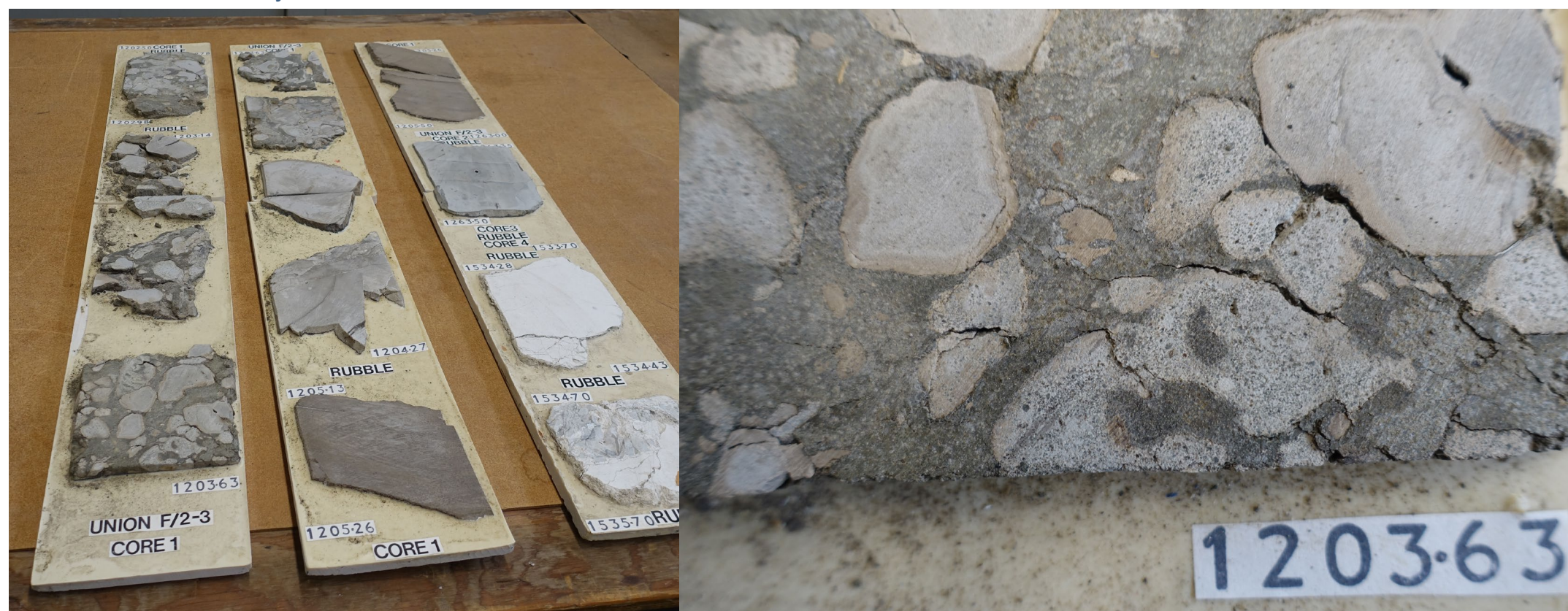
Figure 4.15: Left: Core cut around the MMU in well F02-03. Right: Close-up at 1203.63 m. Badly sorted glauconitic sandy shale with large rounded micritic limestone clasts. Note the yellowish crust around the limestone clasts. Irregularly distributed brownish stain is caused by bitumen.
