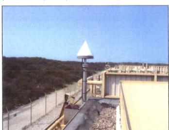
All GPS reference antennas are also surveyed relatively to several nearby height benchmarks by means of levelling, to be able to detect (unsuspected) local subduction of the antennas.
