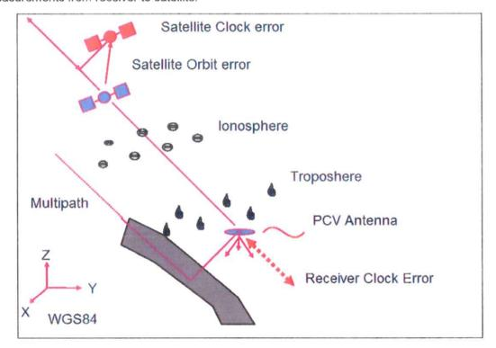
The state space modelling of GNSMART applies beforehand corrections to the GNSS observations. The SSM model is prepared for the following corrections:
