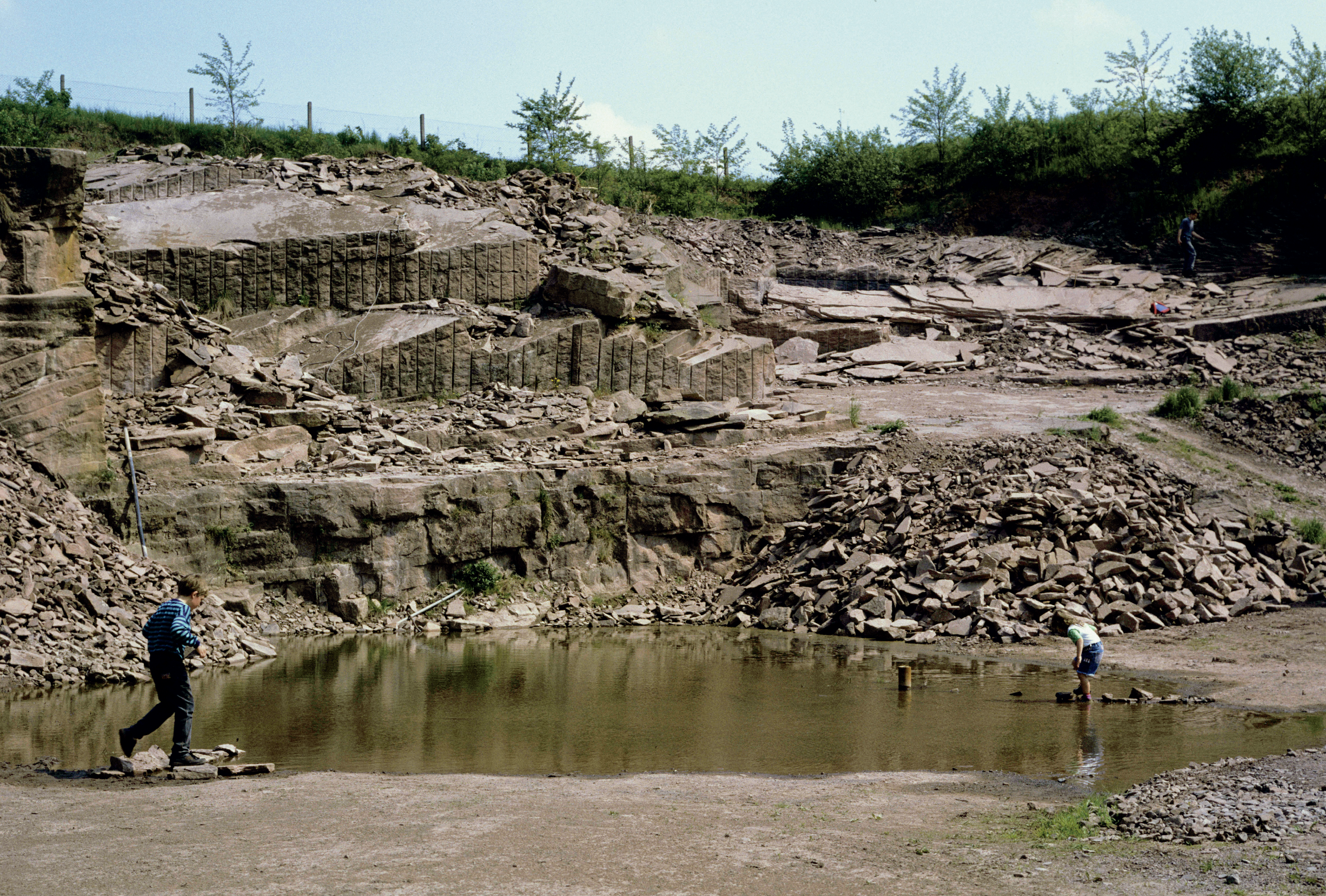
Rotliegend dune-sandstones in the Sventesius quarry at Bebertal, Germany. The grainflow-layers are sold for use as flagstones.
