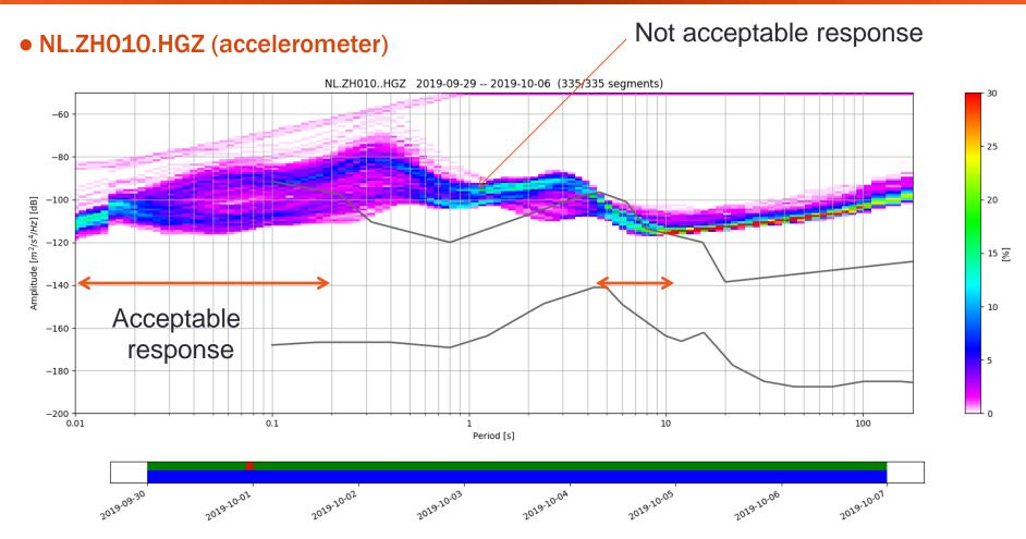
According to the sensor specification: response should be good from 1-2 Hz, which is not the case here. The acquisition has probably derived (which is frequent for long term installations)
