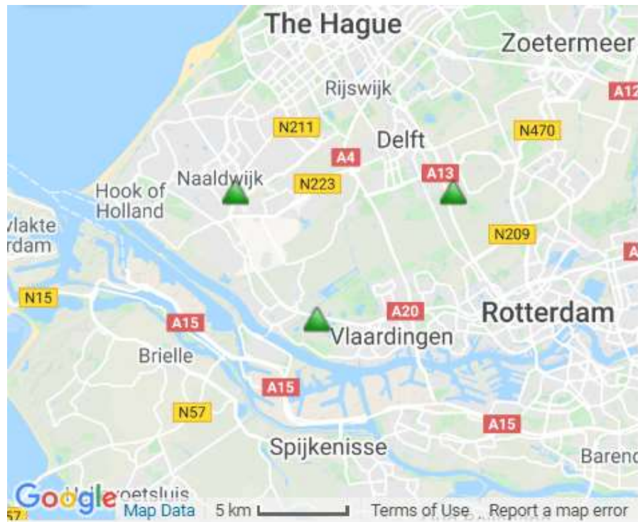
Figuur 15: Seismic stations currently installed in the province of South-Holland (dd 07-2020). Green triangles: ZH01, ZH03, ZH06 wellbore stations (network to be expanded to 10 borehole stations)
