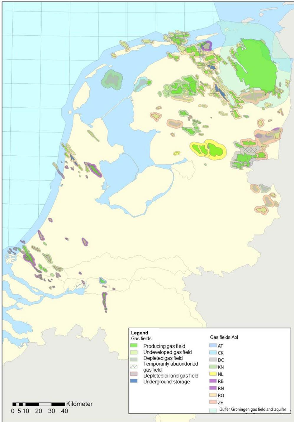
Figure 7 Map showing: 1) Gas fields and gas producing oil fields onshore The Netherlands, 2) Gas field Aol's (coloured by stratigraphic level).
