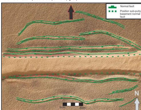
Fig. 62. Top View of model 3 after 75% of the extension phase. The transparent red areas indicate were the silicon putti walls reached the active piercing stage during this stage of the experiment. Both areas will expand slightly futher towards the east during the rest of the experiment. Towards the east, the putti walls will not reach the active piercing stage.
