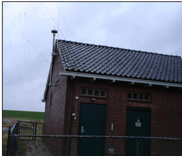
All GPS reference antennas are also surveyed relatively to several nearby height benchmarks by means of leveling, to be able to detect (unsuspected) local deformation of the antennas.
