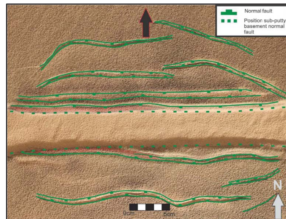
Fig. 62. Top View of model 3 after 75% of the extension phase. The transparent red areas indicate where the silicon putti walls reached the active piercing stage during this stage of the experiment. Both areas will expand slightly further towards the east during the rest of the experiment. Towards the east, the putti walls will not reach the active piercing stage.
