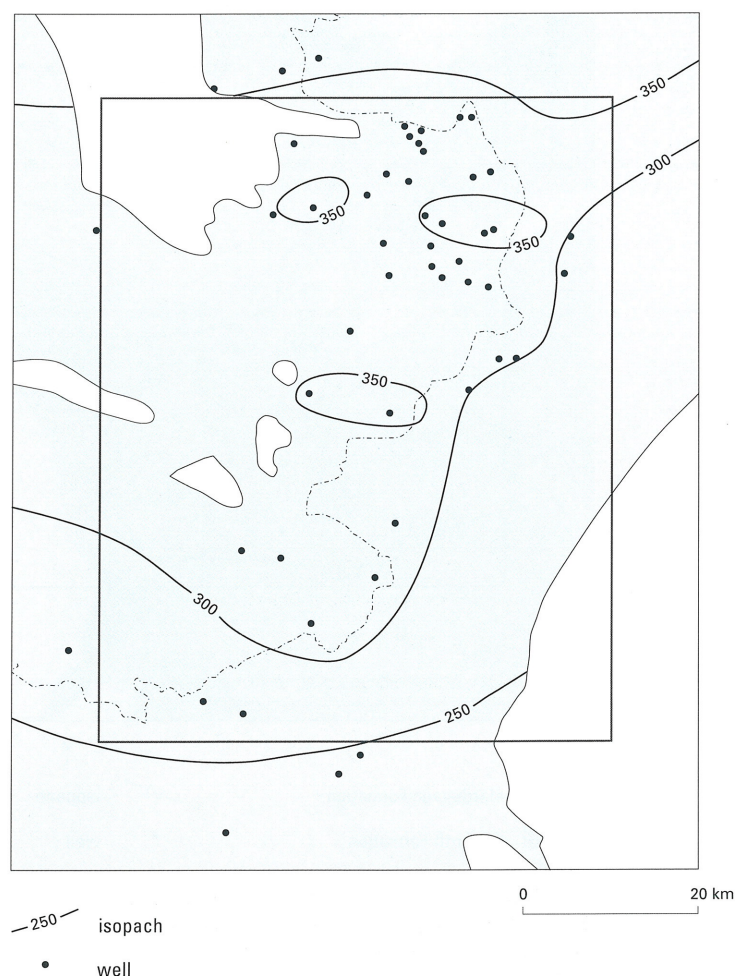
Figure 6.3 Thickness map and extent of the Lower Buntsandstein Formation. The formation thickens in a northerly direction from approximately 275 m to over 350 m in places. This map has been based on well data.
