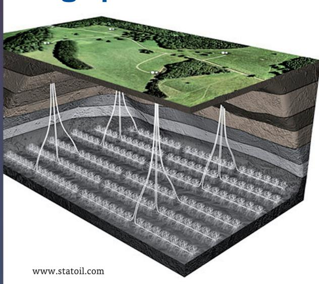
Drilling deviated multiwells from wellpads with downhole multifracs is the most likely concept of developing unconventional resources
