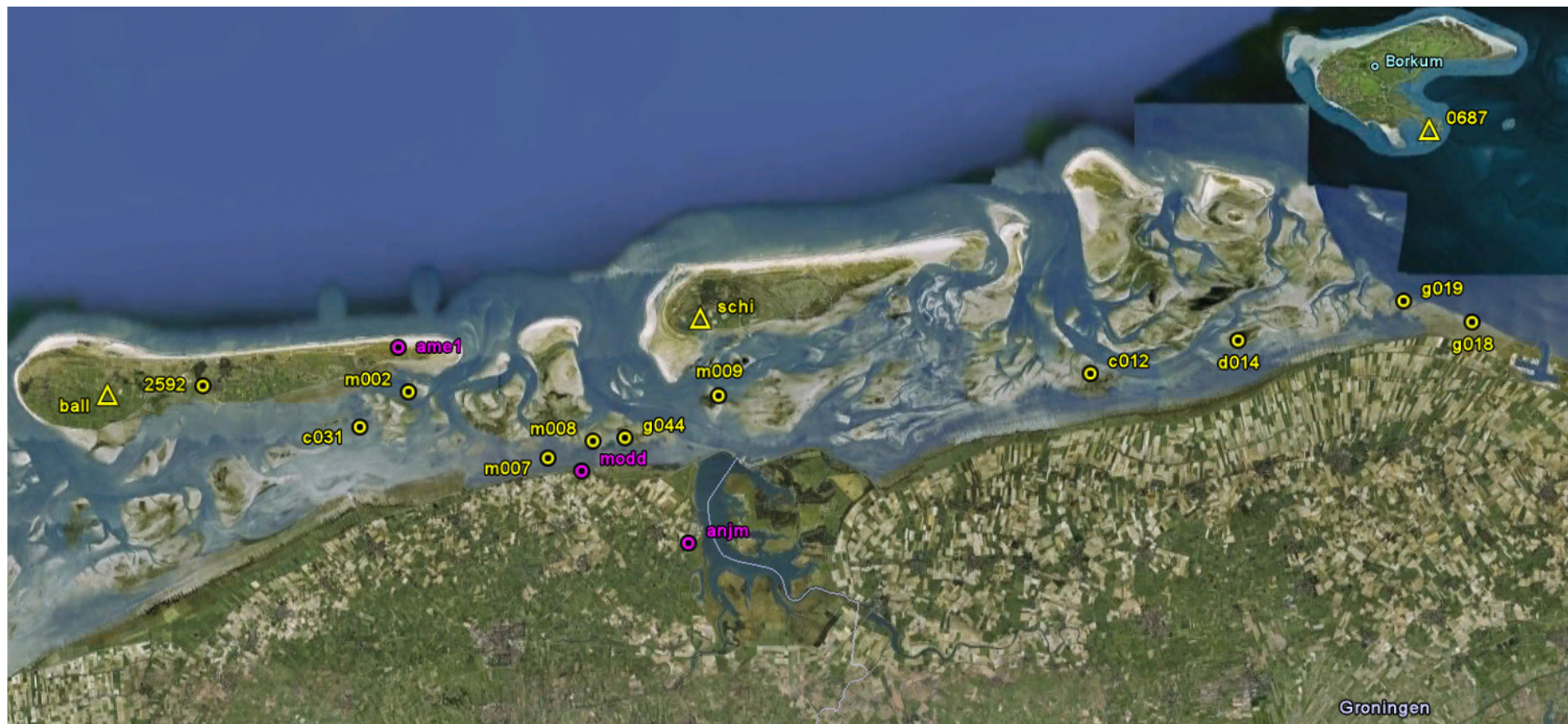
GPS campaign 2010; benchmarks Waddenzee (yellow points), continuous monitoring stations (purple points) and reference stations (yellow triangles)
