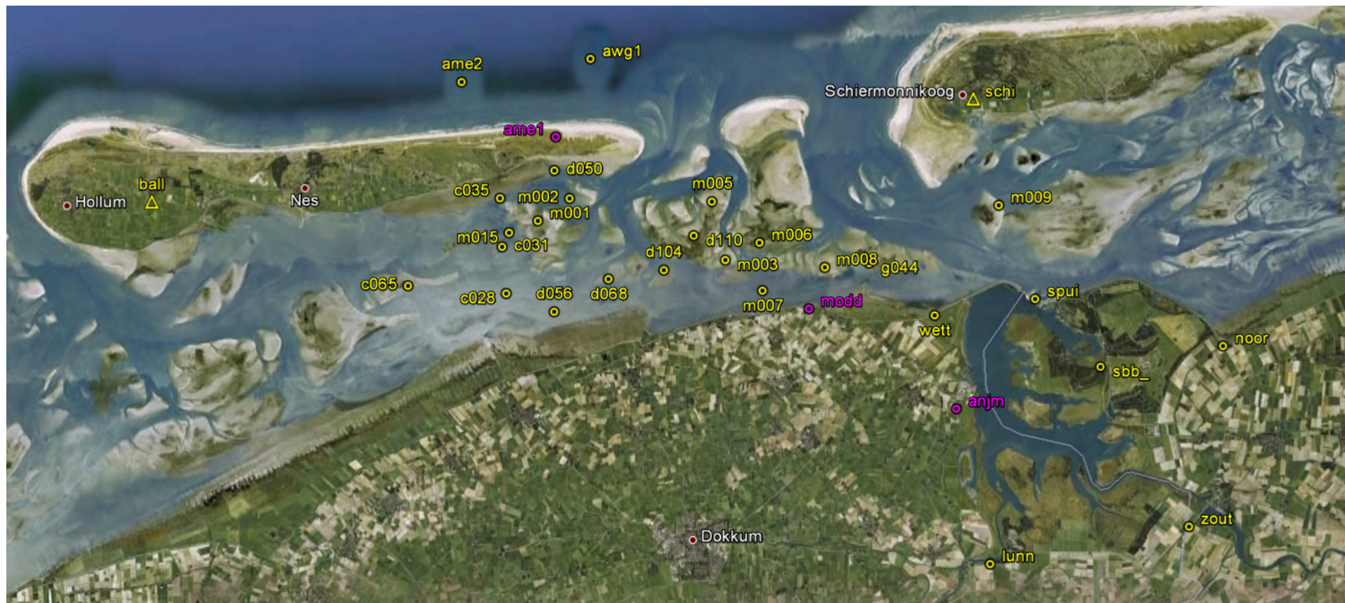
GPS campaign 2011; benchmarks Waddenzee (yellow points), continuous monitoring stations (purple points) and reference stations (yellow triangles)
