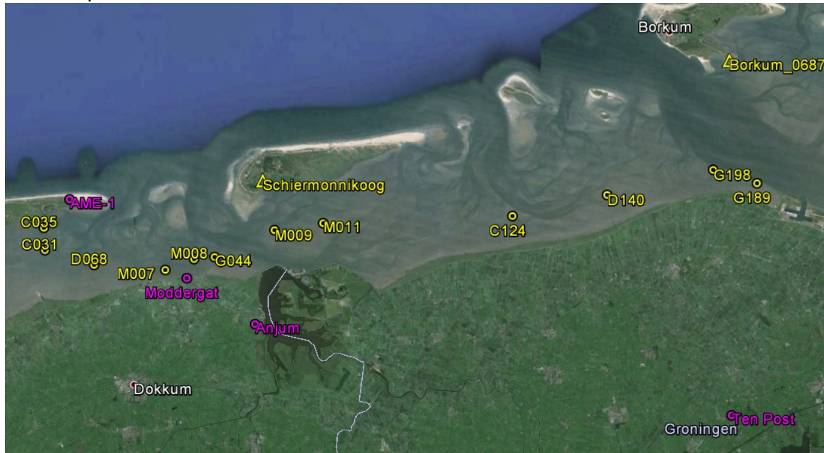
GPS campaign 2013; benchmarks Waddenzee (yellow points), continuous monitoring stations (purple points) and reference stations (yellow triangles)
