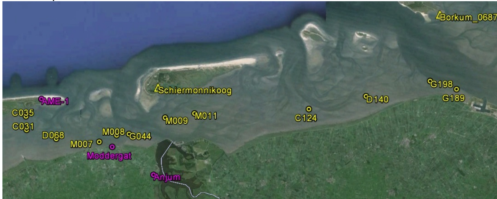
GPS campaign 2013; benchmarks Waddenzee (yellow points), continuous monitoring stations (purple points) and reference stations (yellow triangles)
