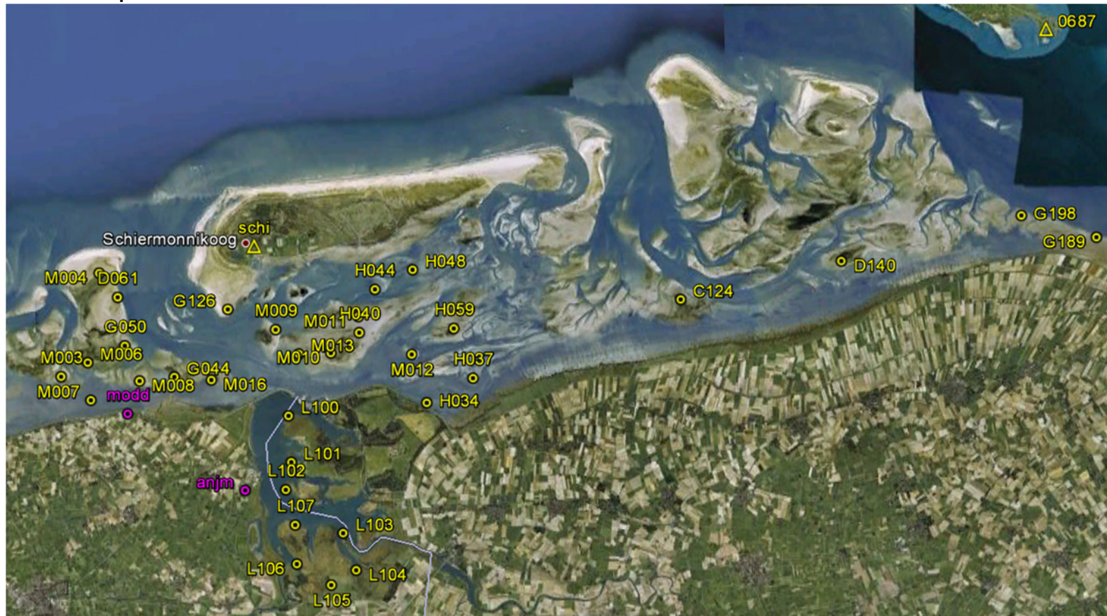
GPS campaign 2012; benchmarks Waddenzee (yellow points), continuous monitoring stations (purple points) and reference stations (yellow triangles)
