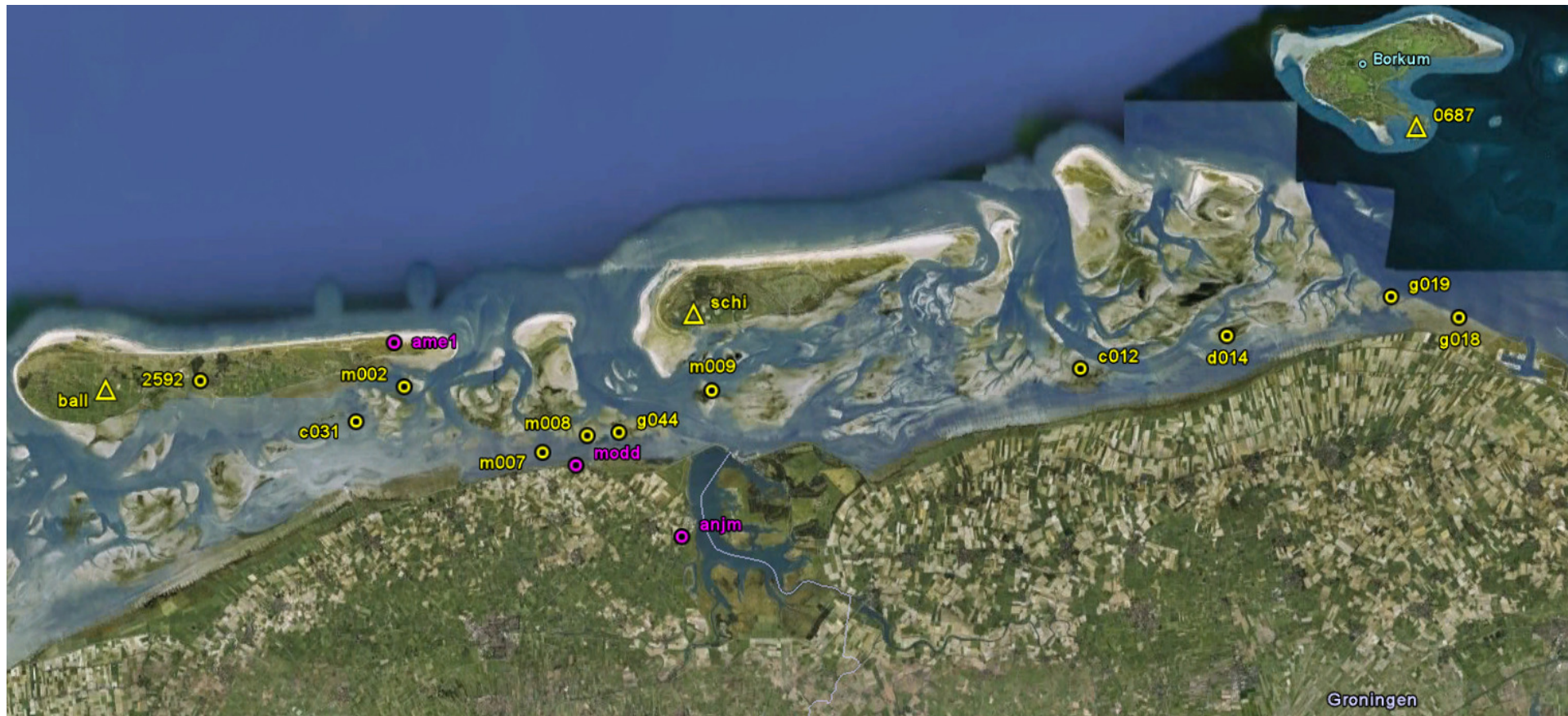
GPS campaign 2010; benchmarks Waddenzee (yellow points), continuous monitoring stations (purple points) and reference stations (yellow triangles)
